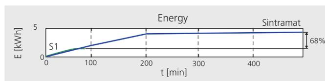
Fig. 4: Energy consumption during the sintering process
