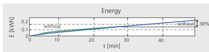
Fig. 3: Energy consumption curve with and without IPF.
